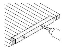
It is advisable to drill small weep holes every 12 inches the bottom "U" profile for condensation drainage.
